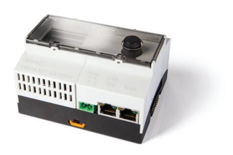
The STRAND VISION.NET GATEWAY is an expandable network gateway for the Vision.Net network, designed to coordinate events between Vision.Net devices using a built-in astronomical clock and NTP server that ensures all devices work from a single timeclock. And because the Vision.Net Gateway is DIN rail mountable, integrators can easily install it in a variety of locations
